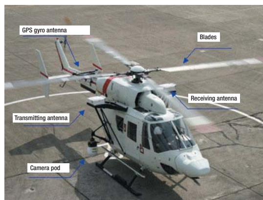
Helicopter equipped with communications equipment and camera
