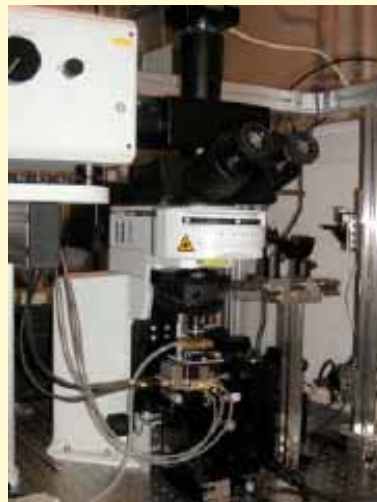
A Photo of polymer-element fabrication instrument. This instrument with simple configurations is capable of creating high-precision polymer-elements on the order of 100 nanometers.
