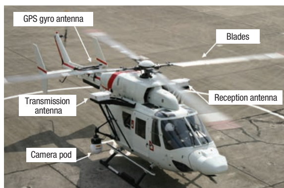
Helicopter standing by at the Gifu airport with the onboard satellite communication system
