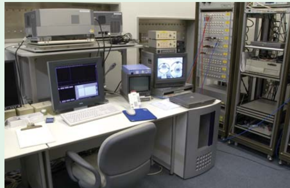
Photo 3. A magnetically shielded operation room for the fMRI, from which various experiments are controlled
