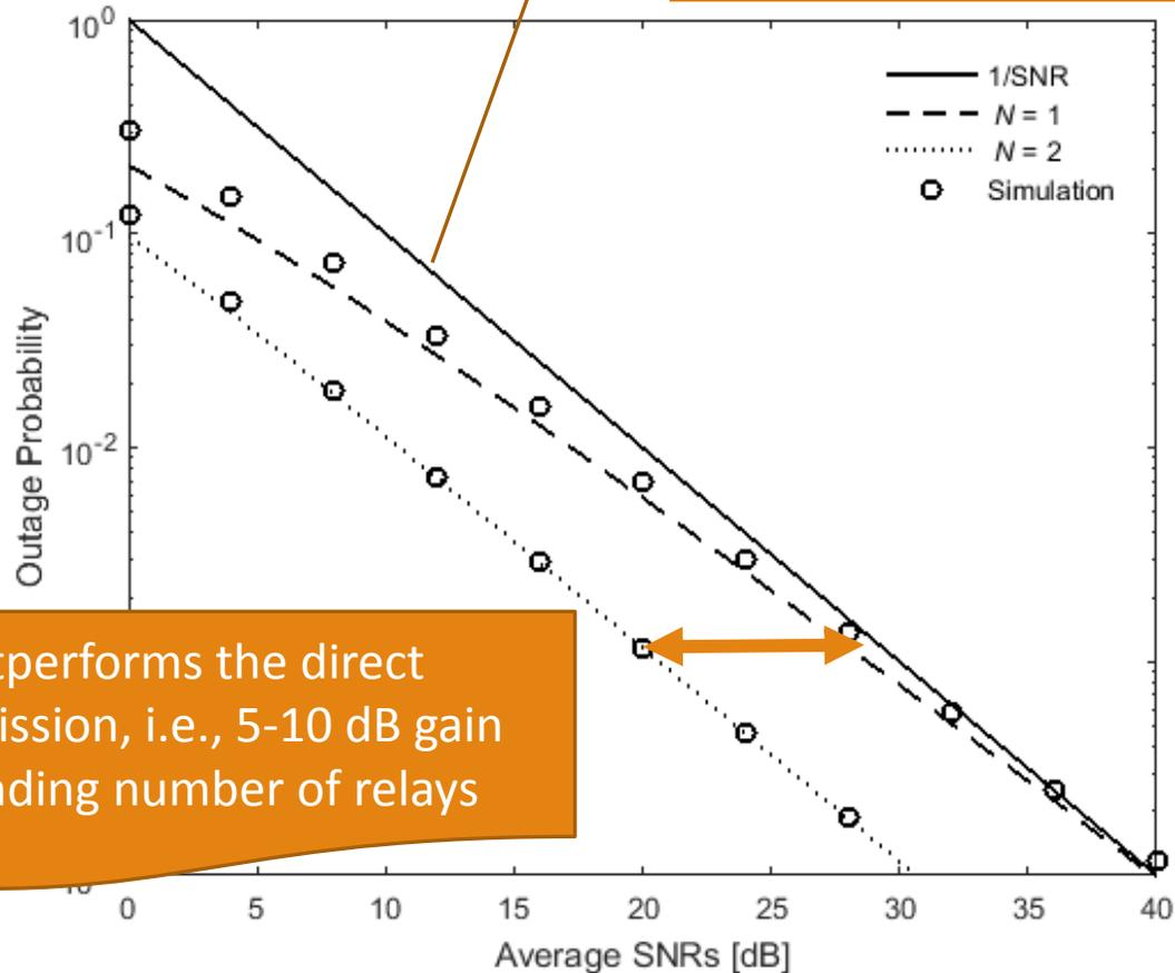
Outperforms the direct transmission, i.e., 5-10 dB gain depending number of relays
