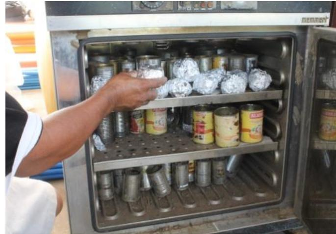
Oven Drying of Soil Sample, overnight at 105 °C (12-24hrs)
