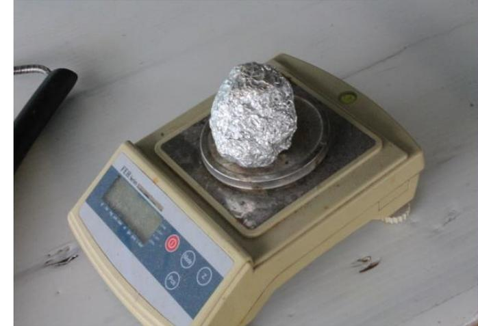
Weighing of Oven Dried Soil Sample
