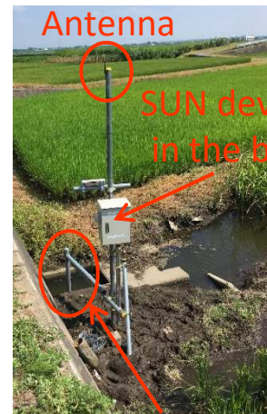
Water level sensor Water management tests in the laboratory and in the rice field
