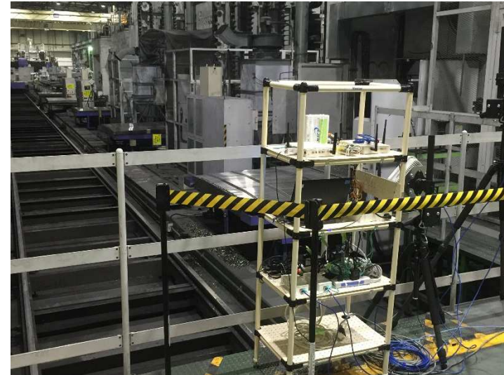
Experimental setup for radio signal monitoring in the factory
