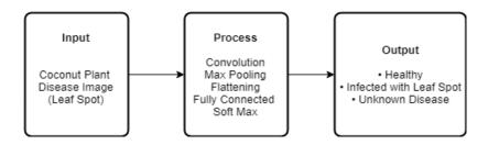
The input is taken from the sample image of a coconut plant disease using the Raspberry Pi camera. The next step is to train the system to identify each image presented to it in the Convolutional Neural Network (CNN) with its extracting features correlated with Python. After training the system and extracting specific features of the leaf spot, the output will be based on the specific features of the leaf spot and classify it whether its diseased, healthy or unknown disease.
