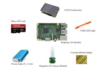
The camera will capture the coconut leaf or stem, with the captured image being sent to the Raspberry Pi module where the processing will be done. It will then be compared to the stored data of the neural network in the micro storage device. The Asus power bank will serve as the power supply with 2.4 Amperes meeting the required current needed to power up the Raspberry Pi module. An LCD touchscreen will be used as the output to show the classification of the image presented.
