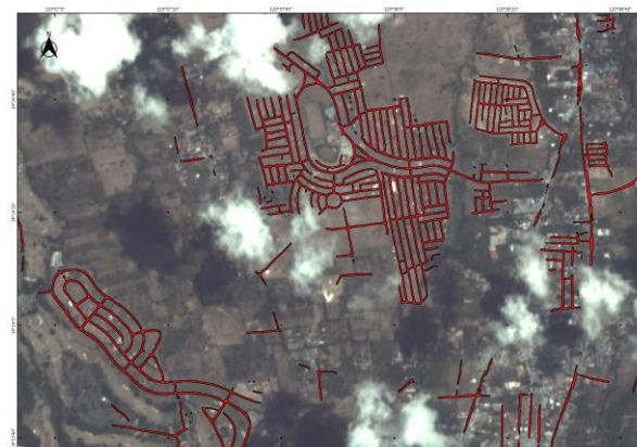
Map Information This map shows the classified roads in an urban area in Slang Cavite. The roads were derived from a 3m resolution Planet satellite imagery taken on April 30, 2018. ROAD DETECTION Using Neural Networks Data Sources Planet satellite imagery provided by the Philippine Earth Data Resource and Observation (PEDRO) Center. Legend Detected Roads using AI 0 250 500 750 1000 m
