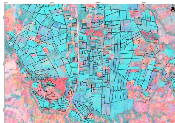
Map Information This map shows the classified sugarcane areas in a portion of Conception, Tarlac. The sugarcane areas were identified using C-band radar images. The map is still subject to validation and the interpretation of remote sensing experts. SUGARCANE DETECTION Using Dynamic Time Warping Data Sources Sentinel-1 images retrieved from the European Space Agency (ESA) Copernicus Open Access Hub ( https://scihub.copernicus.eu/ ). Legend Classified Sugarcane Areas Validated Sugarcane Areas 0 500 1000 1500 2000 m
