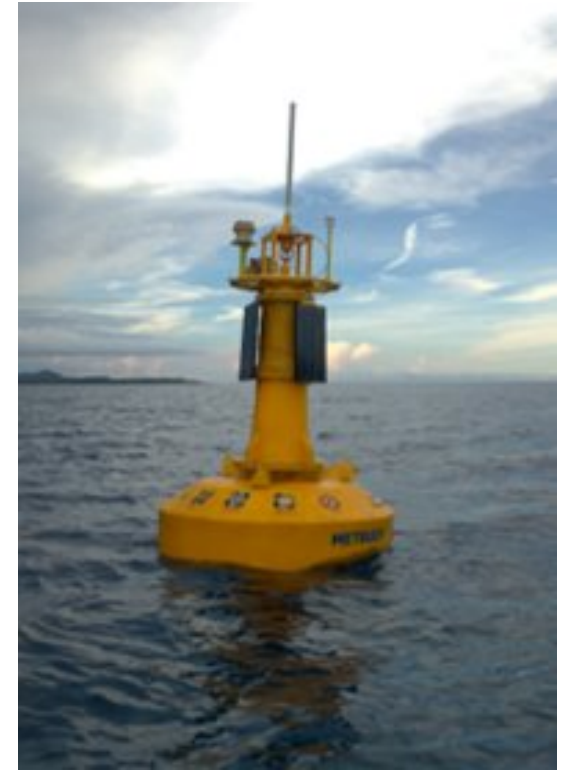
DOST-ASTI developed Communication Relay Buoy
