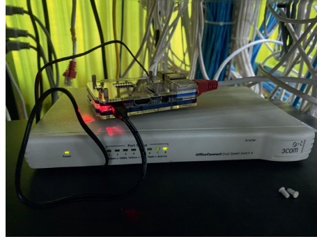
FIGURE 3: Monitoring device (raspberry-Pi 3B) deployed to a LAN.
