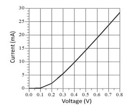
I-V characteristic of the SMS7630 diode
