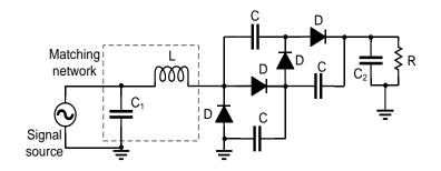
Schematic of a rectifier consisting of a matching network and a two-stage voltage doubler circuit using two zero-bias SBD diodes (SMS7630)
