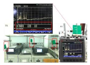
Realistic experiment for testing antenna
