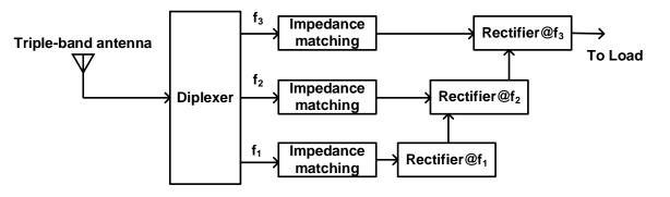
Figure 1. Schematic diagram of the proposed RFEH circuit.
