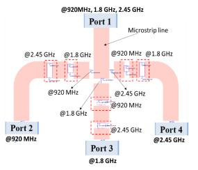
Co-simulation model for the designed diplexer. Total size of this circuit is  $1.8 \text{ cm} \times 2 \text{ cm}$
