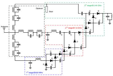
Schematic of the entire RF-EH circuit.
