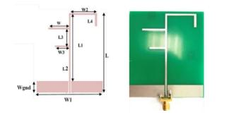
Triple-band antenna: Layout in ADS (left) and fabricated prototype (right).
