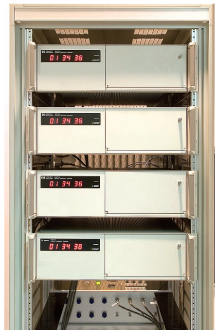
Figure 4 The cesium atomic clocks that form the basis for Japan Standard Time
