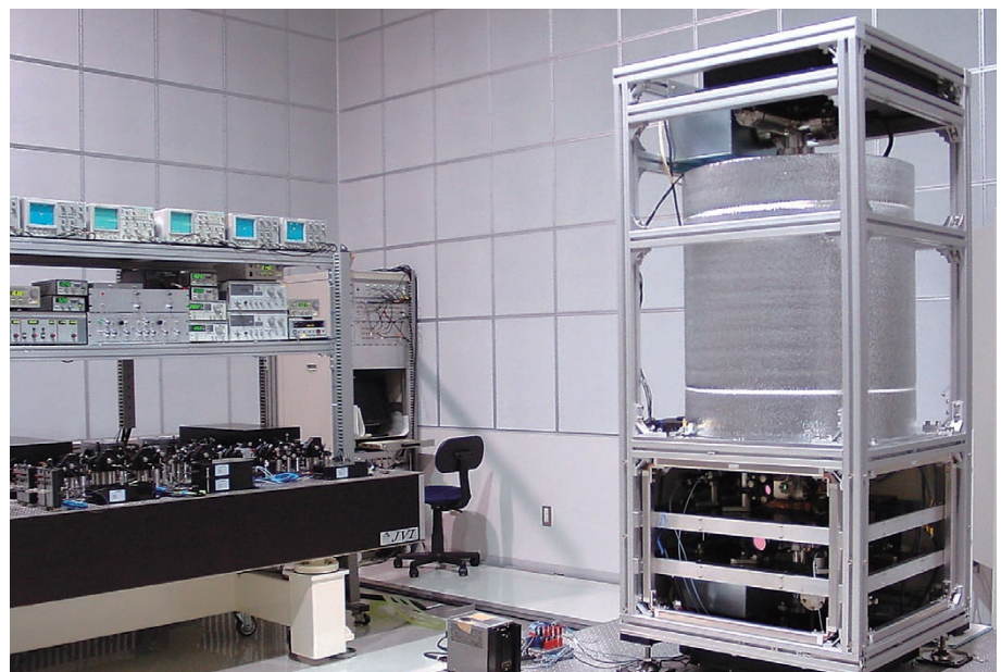
Figure 2 NICT-CsF1 cesium fountain primary frequency standard
