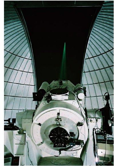
Figure 3 1.5 m telescope satellite laser ranging
