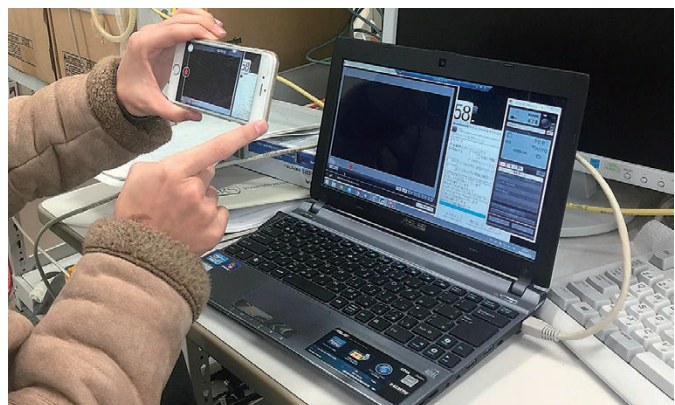
Figure 6 Portable telescope observation system not using any special devices. (Using a smartphone to photograph the screen of the PC to record the experimental process.)
