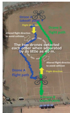
Figure 3 Autonomous flight control field test using two drones
