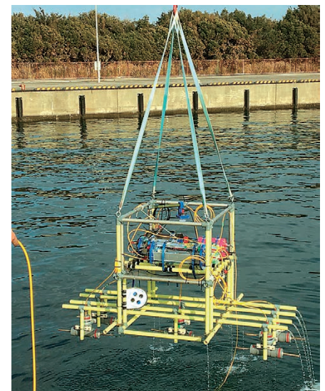
Figure 3 Sensing and measurement frame equipped with one transmitting antenna and four receiving antenna arrays
