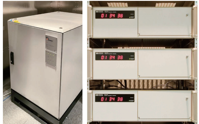
(Left) Hydrogen maser clock
