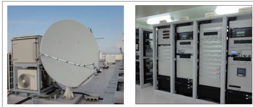
Fig.1 : The Japan Standard Time system at the JST sub-station at Kobe(left: Antenna of satellite time comparison system, right: Measurement system)
