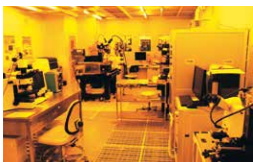
Photo-lithography equipments in the clean room with yellow lights
