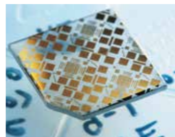
Chip fabricated with Ga 2 O 3 transistors and diodes
