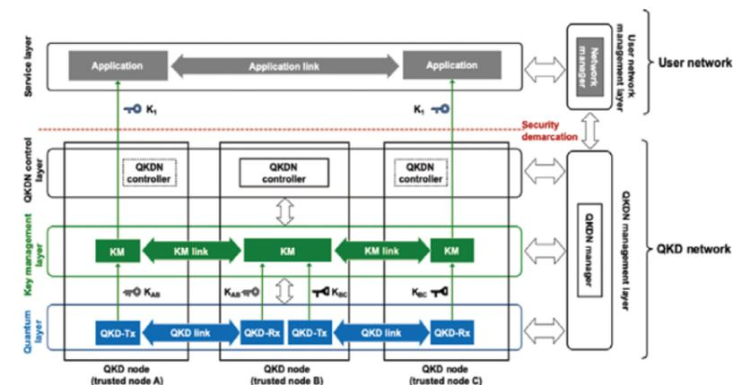
Figure 2 Basic configurations of the QKD network and user network specified in the international standard recommendation, ITU-T.Y.3800
