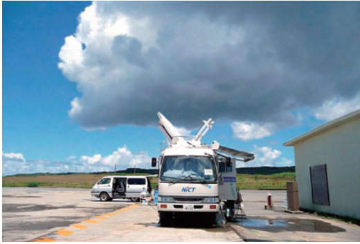
Figure 3: NICT Land Mobile Station Used in an Environment Spewing Sulfur Gas after an Intense Squall Affecting the 28 GHz Uplink
