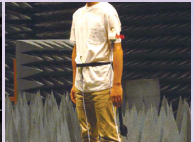
Figure 3: A View of Taking Measurements for Modeling Radio-wave Propagation around a Human Body
