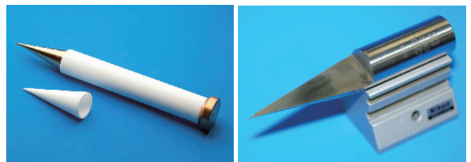
Figure 5 ● Teflon coating (white part) side diameter 36 mm, full length 325 mm and a tool made in-house to bore the cone
