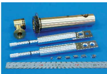
Figure 3 ● Specimen Holder for Terahertz Spectroscopy (Full length 255 mm)
