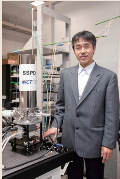
Figure 4 ● Superconducting Photon Detector The use of superconducting photon detector enhances photon detection efficiency and reduces noise level. This is an indispensable apparatus for long-distance and high-speed quantum cryptography.
