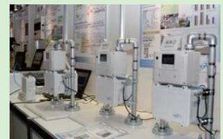
Prototype of a smart meter with low-power radio devices, which conforms to IEEE802.15.4g/4e and enables the service coverage to expand by means of multi-hop communications. We also demonstrated its connection to a radiation dosimeter.
