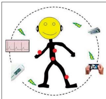
Figure 1 ●BAN that connects various small devices placed in the vicinity of, or inside of, a body
