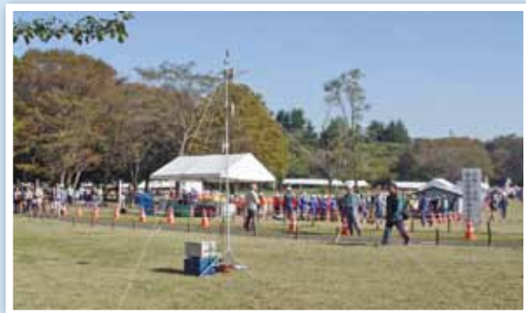
●NerveNet base stations installed in various locations in Koganei Park Using directional planar antennas, we installed the stations at intervals of 200 to 300 m.
