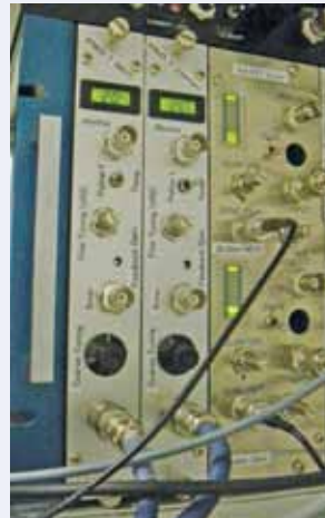
Figure 1 ●A housing that I made for an electrical circuit (NIM unit for temperature control circuit)
