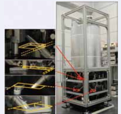
Figure 2 ●Primary frequency standard NICT-CsF2 (right) and breadboard processed around the trap part Area in yellow indicates notched parts.
