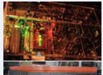
Figure 3 ●Optical comb (upper) and side of resonator cover (Orange acrylic board is 5 mm thick)
