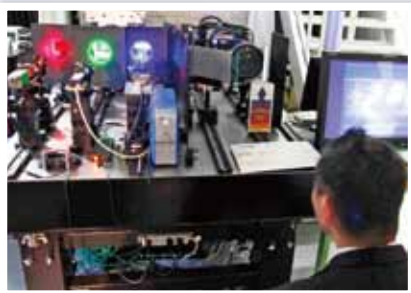
● Electronic holography using display elements at 8K resolution (16x a household television)
