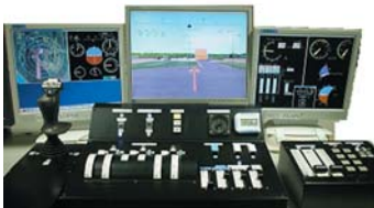
Figure 3: Airship flight controller (CG screens are created by FLOPS)
