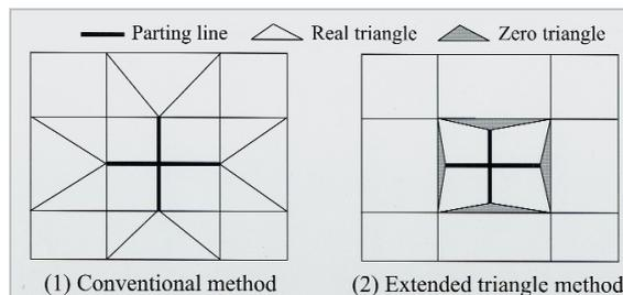
**Fig.8** Mesh subdivision processing based on extended triangles
