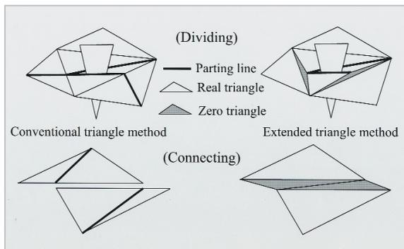
**Fig.5** Extended triangle geometric processing
