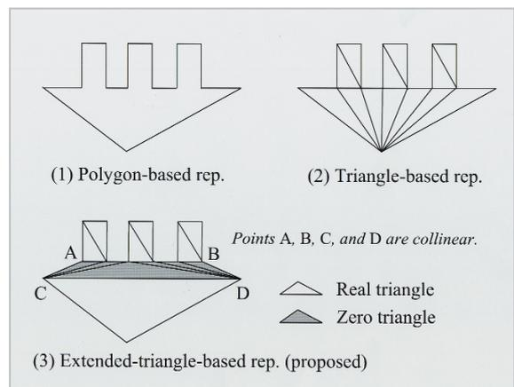
**Fig.4** Extended-triangle-based representation
