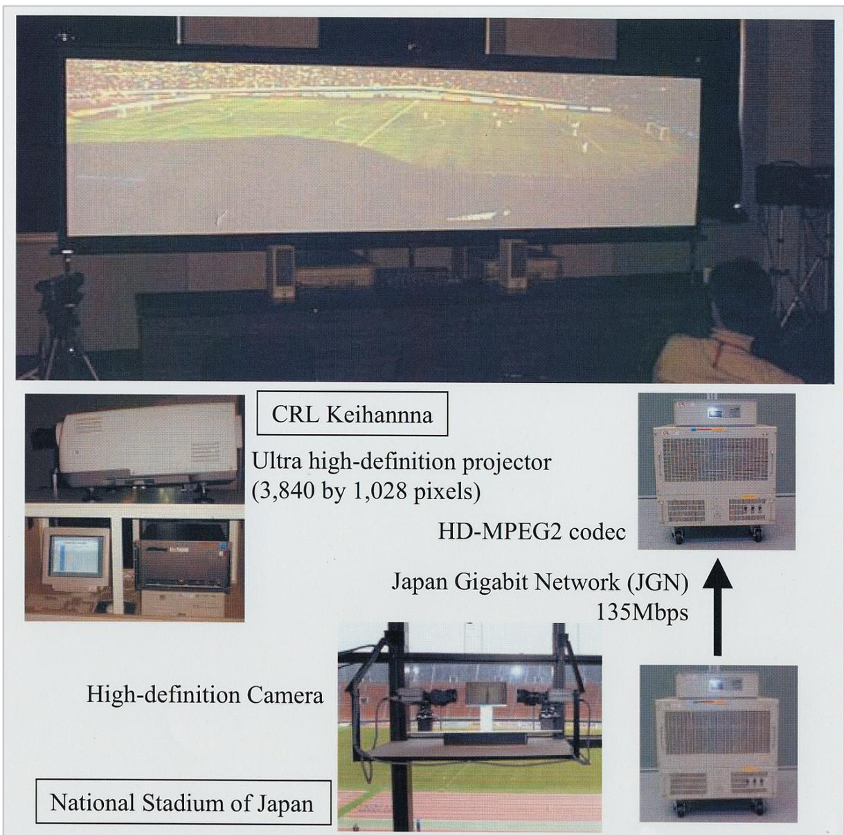
**Fig. 14** An ultra high-definition image transmission experiment on the first day of the 21st century
