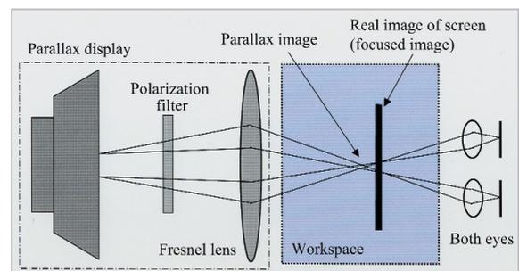
**Fig.10** Stereoscopic display method that simultaneously uses both parallax and focus
