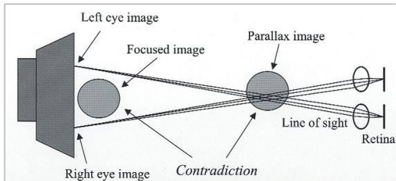
**Fig.9** Stereoscopic display method based only on parallax
