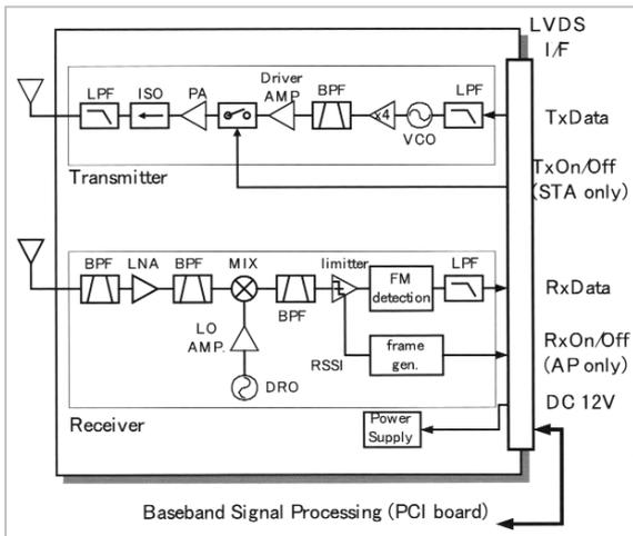
**Fig.5** Diagram of transceiver
