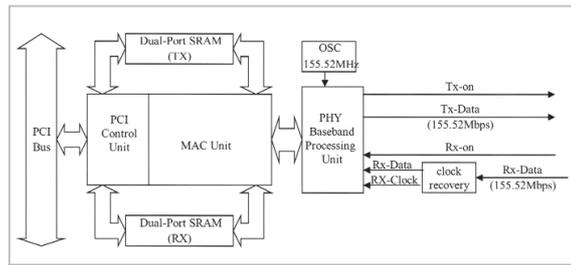
**Fig.7** Block diagram of DLC board
