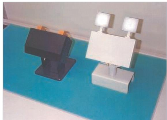
**Fig.4** Photo of transceivers (left: STA; right: AP)
