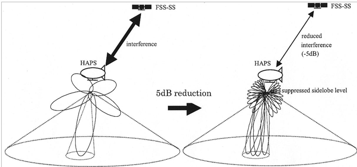
**Fig. 10** Radiation pattern improvement by beam-shaping
