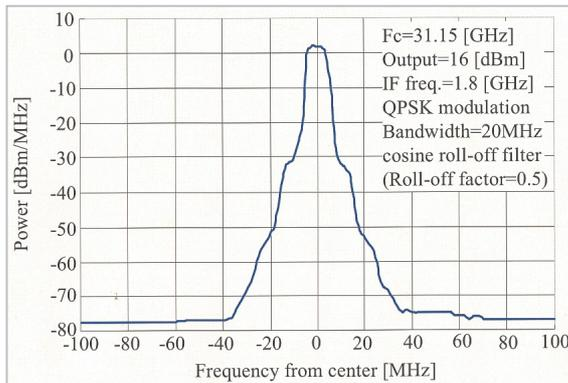
**Fig.9** Measured spectrum (per 1 MHz) of the output signal emitted from the developed 31 GHz-band RF module
