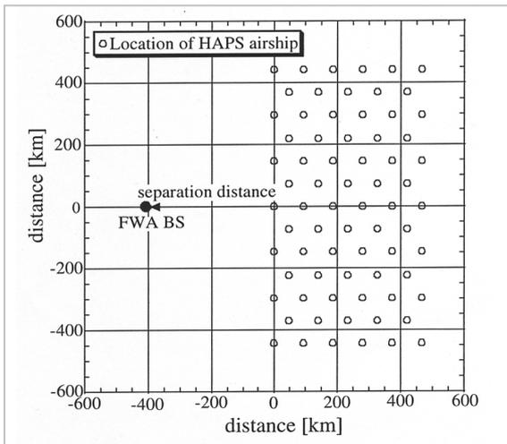
**Fig. 6** 11 x 21 HAPS airships deployed in 500 km x 1000 km area
