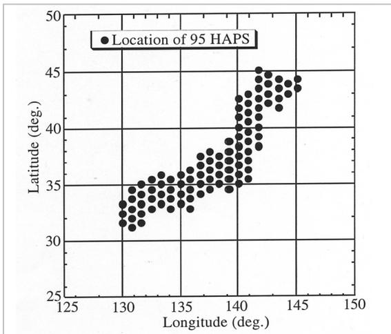
**Fig.2** Example of HAPS deployment for stratospheric platform system in Japan (assuming a minimum elevation angle = 20 degrees)
