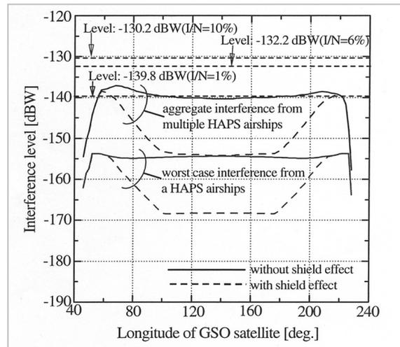
**Fig.4** Interference with GSO-FSS satellites caused by the HAPS downlink
