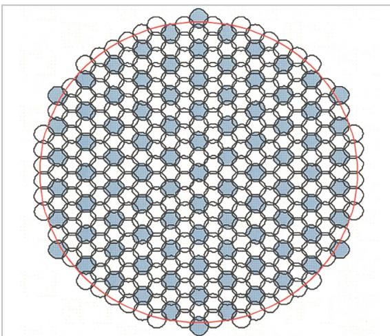
**Fig.3** Example of terrestrial footprints formed by an airship (minimum elevation angle = 20 degrees; 367 cells)
