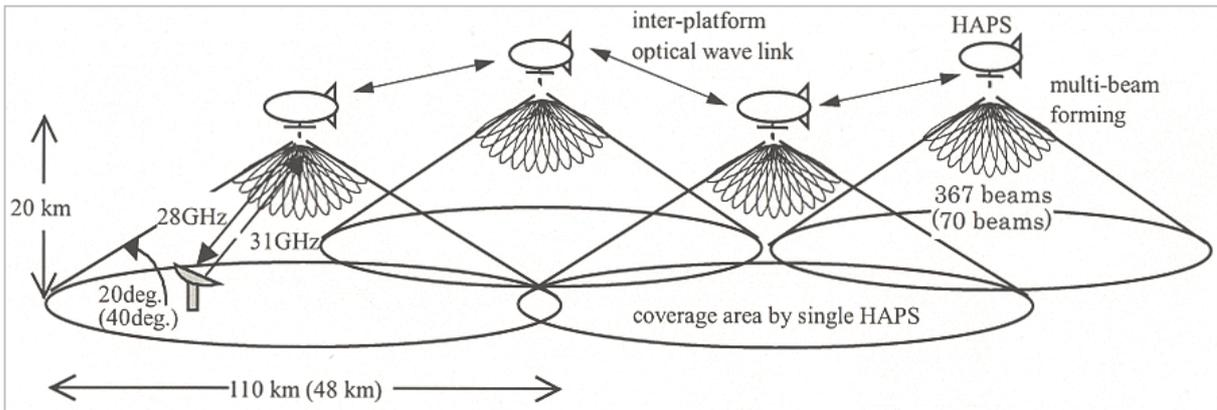
**Fig. 1** Schematic illustration of the Ka-band wireless communications system for fixed service using the stratospheric platform
