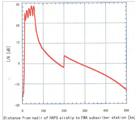
**Fig. 8** I/N characteristics in the FWA substitution with regard to interference caused by one HAPS station
