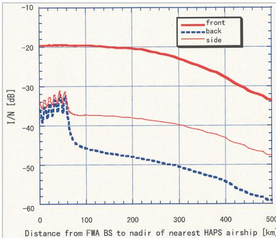
**Fig. 7** I/N characteristics of interference with the FWA hub station caused by the 11 x 21 HAPS airships
