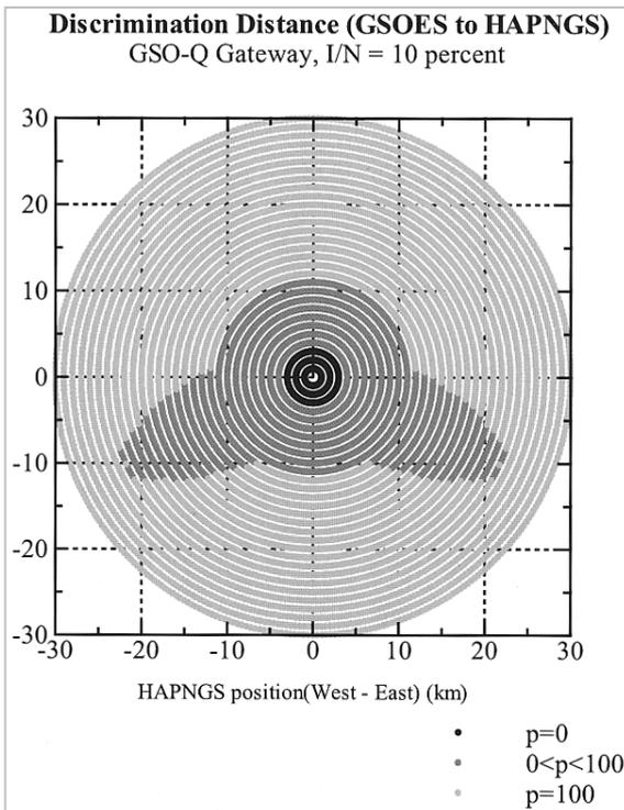
**Fig.5** Probability for deploying HAPS ground stations (the center is the GSO-FSS earth station)
