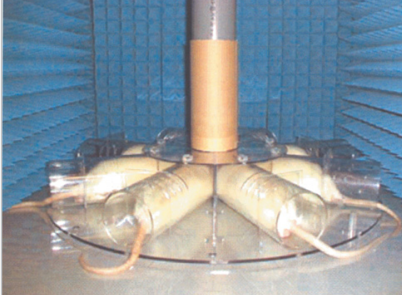
Fig.5 Rat-brain localized exposure setup
