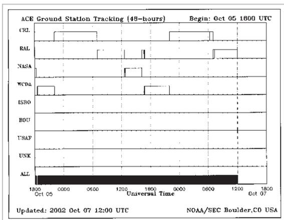
**Fig. 1** Task chart of ACE/RTSW ground receiving stations
