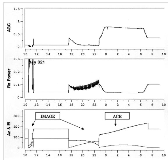
**Fig.5** Record of 24-hour spacecraft tracking using the 11-m antenna
