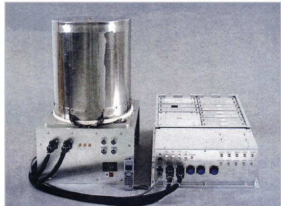
Fig.3 Breadboard model of space-borne micro hydrogen maser
