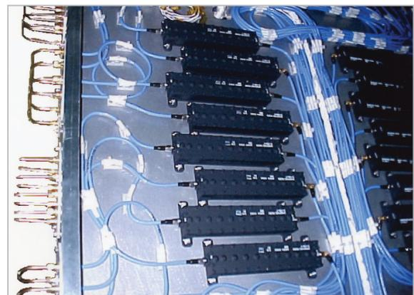
**Fig.4** Filter arrangement in Rx unit
