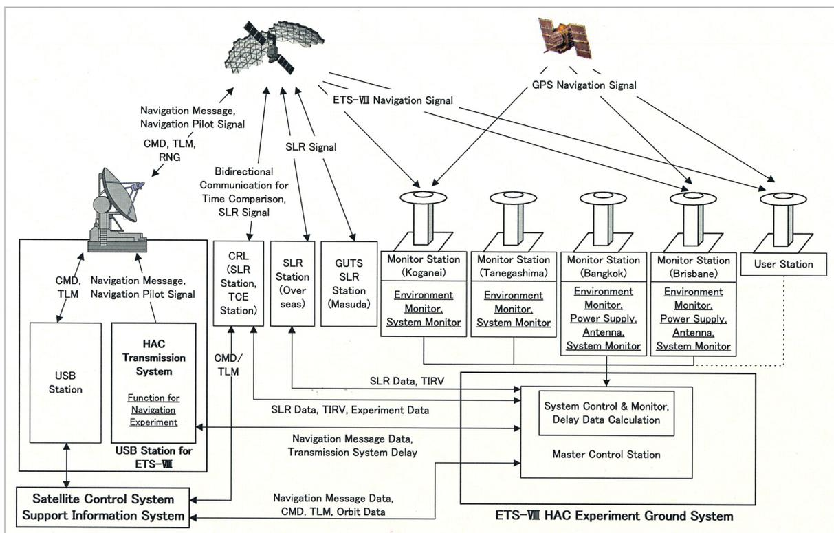
Fig.5 ETS-VIII satellite positioning experimental system
