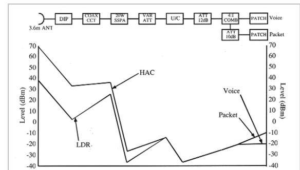
**Fig. 13** Level diagram of transmitting system
