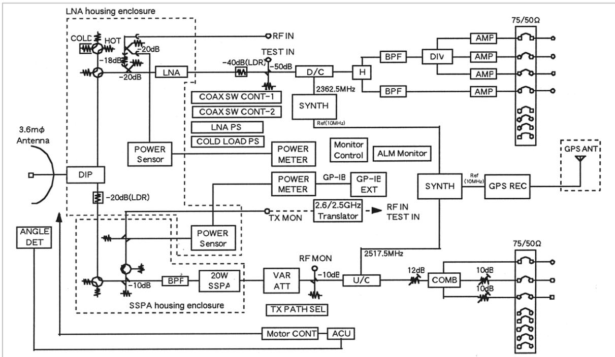
**Fig.1** Block diagram of S-band earth station
