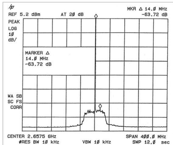
**Fig.9** Spurious of transmitting system
