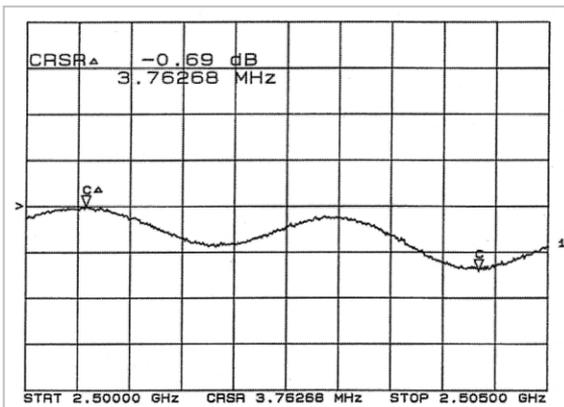
**Fig. 11** Amplitude-frequency characteristics (communication) of receiving system
