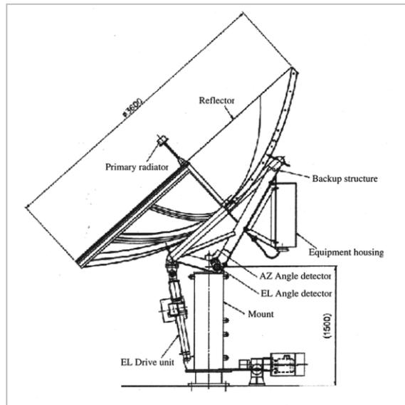
**Fig.3** Appearance of antenna unit
