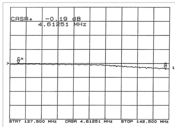
**Fig.8** Amplitude-frequency characteristics of transmitting system
