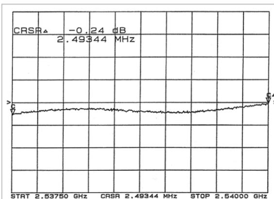
**Fig. 12** Amplitude-frequency characteristics (broadcast) of receiving system
