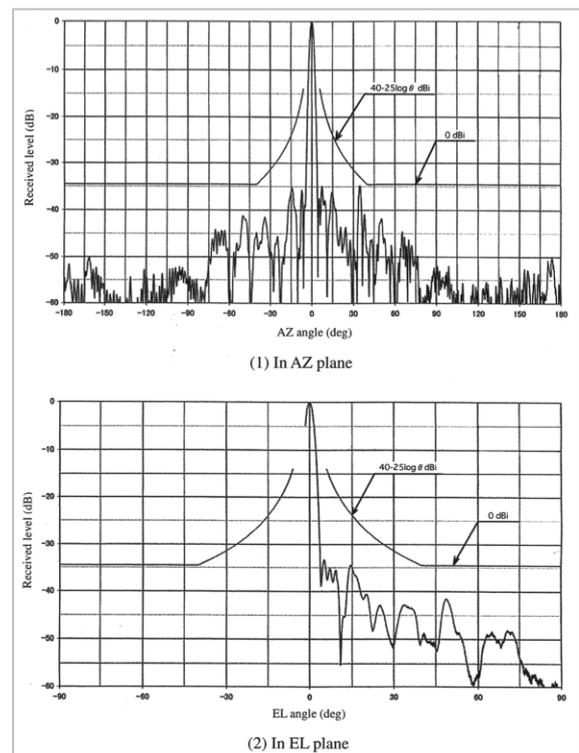
**Fig.5** Receiving antenna pattern
