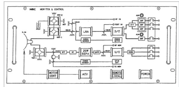
**Fig.6** Front panel of monitor & control device
