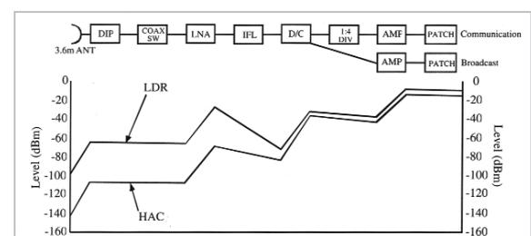
**Fig. 14** Level diagram of receiving system (communication)
