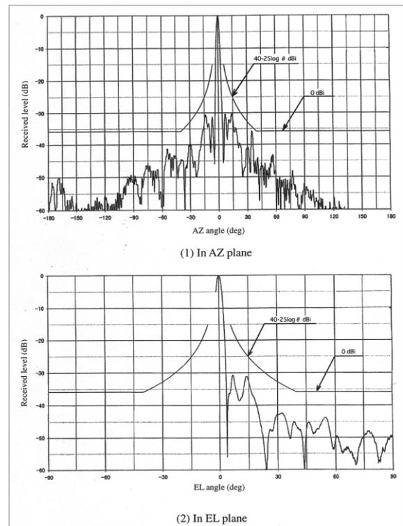
**Fig.4** Transmitting antenna pattern
