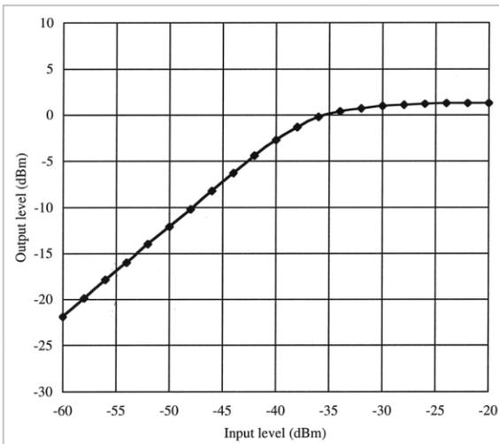
**Fig. 10** Input-output characteristics of LNA
