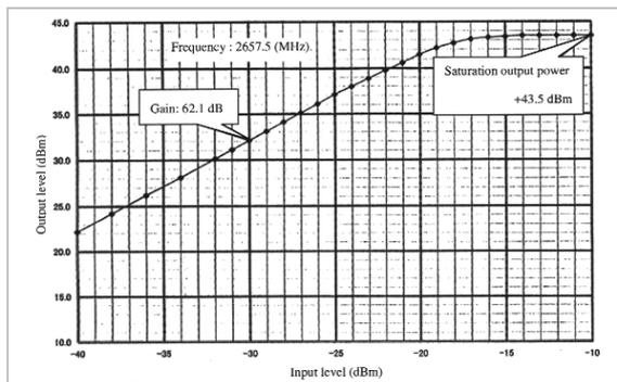
**Fig.7** Input-output characteristics of 20-W SSPA
