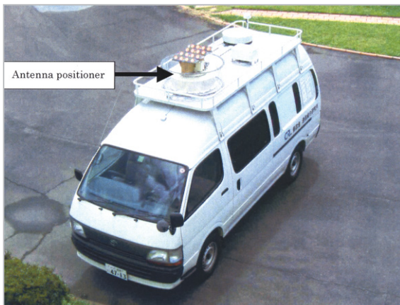
Fig. 1 Appearance of the land mobile station (LMS). An S-band stair-type antenna is mounted on the antenna positioner. The radome has been removed.
