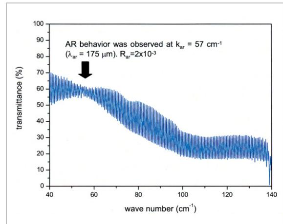
**Fig.3** This figure shows transmittance spectrum of the Ge wafer (1989.5 μm thick) with an AR coating (a 20.9-μm-thick SiO<sub>2</sub> layer) on one surface. The reflectivity of  $2 \times 10^{-3}$  has successfully demonstrated at  $k = 57 \text{ cm}^{-1}$ .
