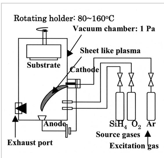
**Fig. 1** Diagram of the plasma enhanced CVD
