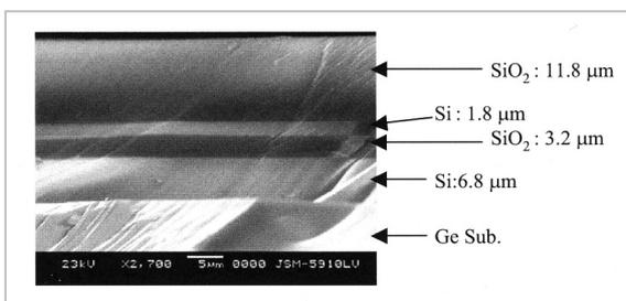
**Fig.4** The SEM viewgraph of the cross section of four layer AR coating
