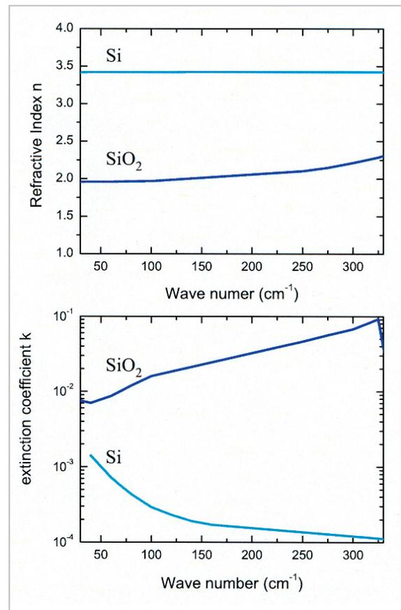
**Fig.2** Optical constants of Si and  $\text{SiO}_2$
