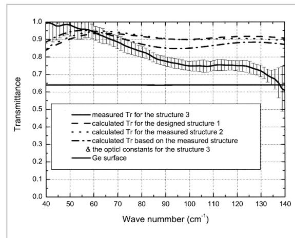
**Fig.6** The calculated transmittance for the structure 1, 2, and 3 are shown by dotted lines. Black solid lines show the measured transmittance for the structure 3 and for the Ge surface.
