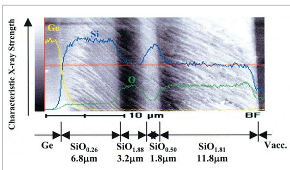
**Fig.5** The cross-sectional SEM viewgraph of the four layer AR coating with the results of EDS analysis
