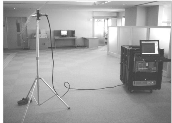
**Fig. 12** Experimental environment for interception using an antenna
