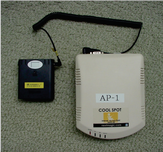
Fig. 16 Wireless LAN access point used in the experiment (powered by an external rechargeable battery)
