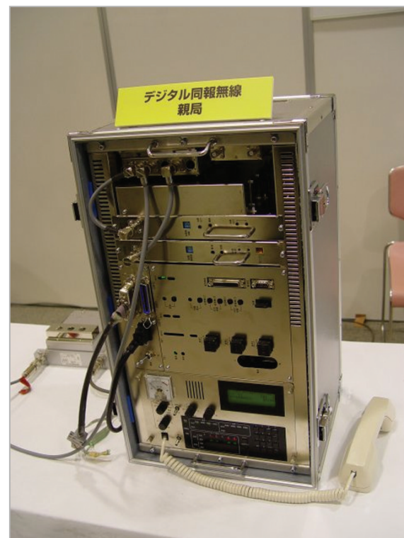
Fig.3b Master radio station at the emergency control center Manufactured by Oki Electric Industry Co., Ltd.
