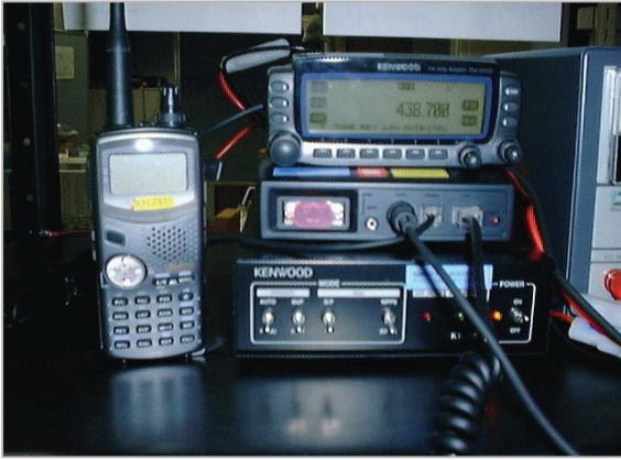
Fig.9 One set of experimental equipment for simple data transmission using an amateur radio to transmit DTMF codes
