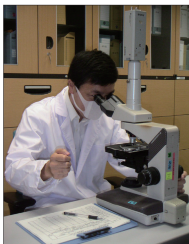
Fig.1 Asbestos fibers measurement based on conventional method (using a hand-held counter)
