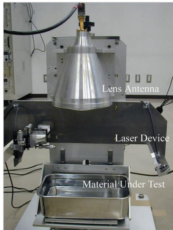
**Fig.6** Biological-body dielectric-constants measurement system using lens antennas
