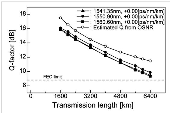
**Fig.6** Transmission characteristics of MD-DMF
