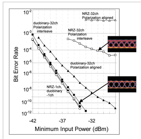
**Fig.2** Bit error rate characteristics of various high-density multiplexing methods for 10-Gbps, 12.5-GHz-interval transmission
