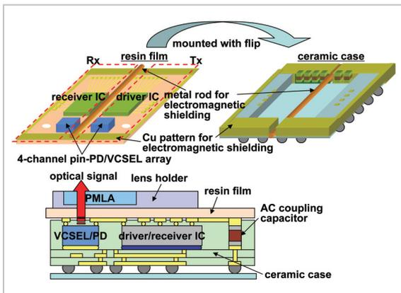
**Fig. 8** Configuration of ultra-small optical I/O
