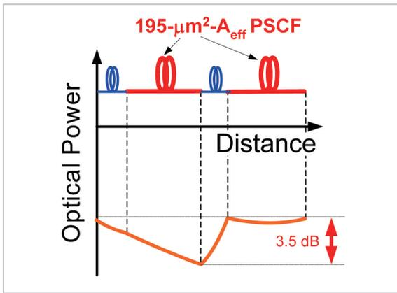
**Fig.3** Configuration of transmission line with low nonlinearity
