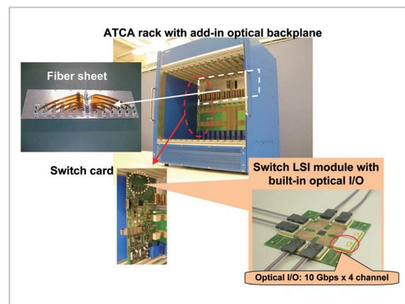
**Fig. 11** Simplified switching system using ATCA standard rack
