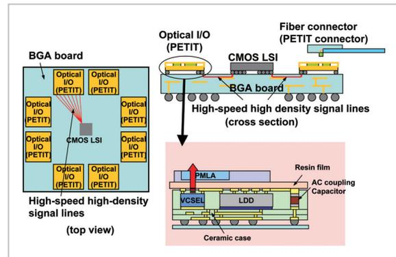
**Fig.7** Conceptual illustration of switch LSI module with built-in optical I/O
