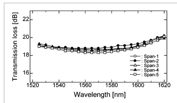
**Fig.5** Loss characteristics of MD-DMF
