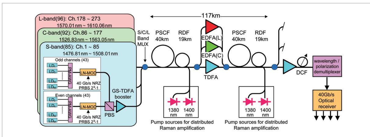
Fig. 1 System configuration of 10-Tbps WDM transmission experiment
