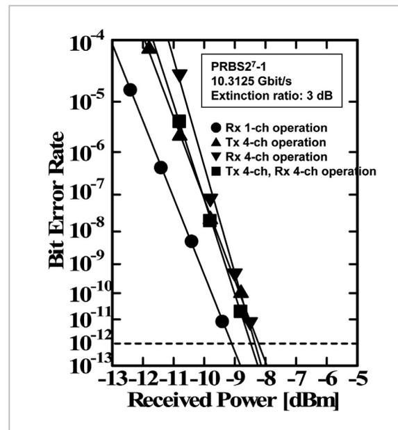
**Fig. 10** Receiving characteristics of optical I/O
