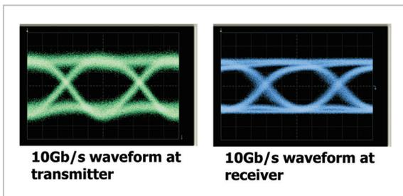
**Fig. 9** Transmitter and receiver waveform of optical I/O
