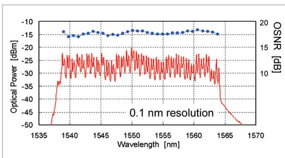
**Fig.4** Optical spectrum after transmission over 9,000 km
