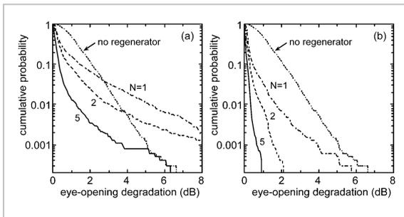
**Fig.5** PMD compensation effect produced by signal regenerator. Cumulative distribution of eye-opening degradation (a) when  $n$  sets of 2R regenerators are inserted into the transmission line and (b) when timing regeneration by synchronous modulation is combined with 2R regeneration
