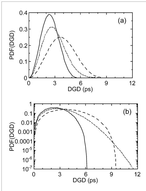
**Fig.3** Probability density function of total DGD for a transmission system consisting of six fibers with fixed DGD. The solid curve represents Set A, the dashed curve represents Set B, and the dotted curve represents the Maxwell distribution. The vertical axis is shown (a) in linear scale and (b) in logarithmic scale.
