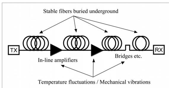
**Fig.2** Model for installed transmission line
