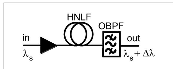
**Fig.4** All-optical 2R regenerator based on nonlinear effects of optical fibers. HNLf: highly nonlinear fiber; OBPF: optical bandpass filter
