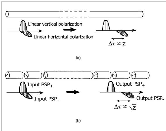
**Fig. 1** Behavior of optical pulses propagating in (a) linear birefringent fiber (polarization-maintaining fiber) with a constant birefringence and (b) general single-mode optical fiber (non-polarization-maintaining fiber). (Despite the explanation in the main text, this figure illustrates pulses input to the fiber instead of a continuous wave.)
