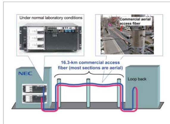
**Fig.4** Experimental configuration
