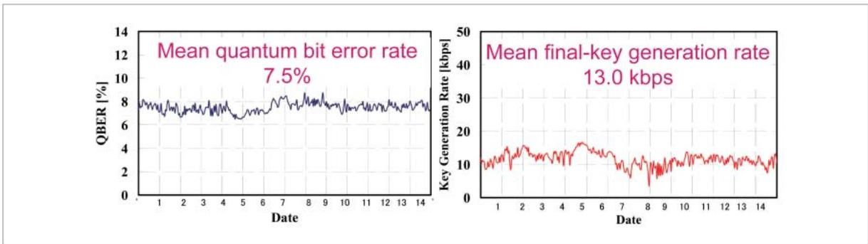
**Fig.5** Transition of quantum bit error rate and final-key generation rate
