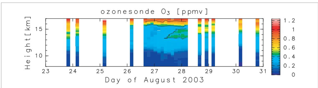
**Fig.3** Time-altitude cross-sectional diagram of the ozone mixing ratio obtained by ozonesonde observation (altitudes of 8–17 km)
