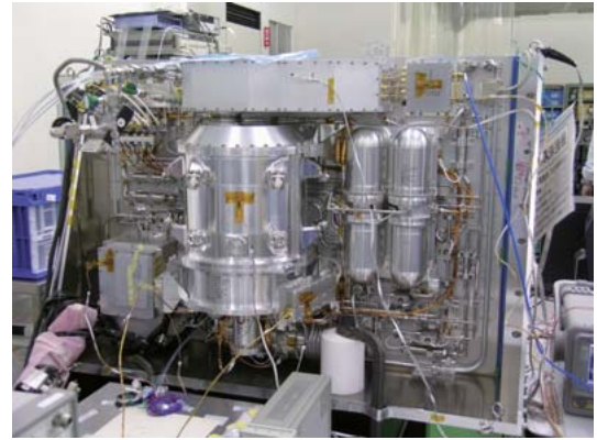
Fig.5 SMILES submillimeter-wave receiver tested for performance
