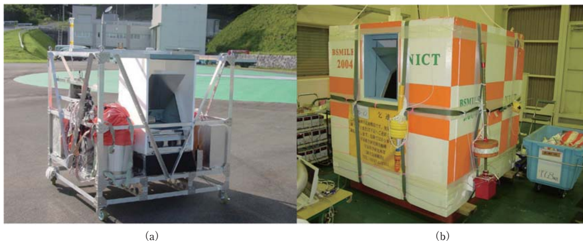
Fig.4 (a) External view of BSMILES and (b) instrument package for launch
