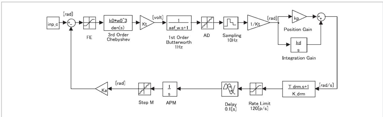
**Fig. 11** Block Diagram of Antenna Pointing System
