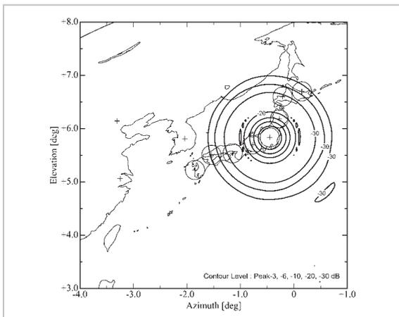
**Fig.3** Antenna Gain Contours of Kanto Beam (TX)
