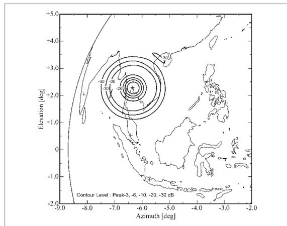
**Fig.5** Contours of Bangkok Beam (TX)
