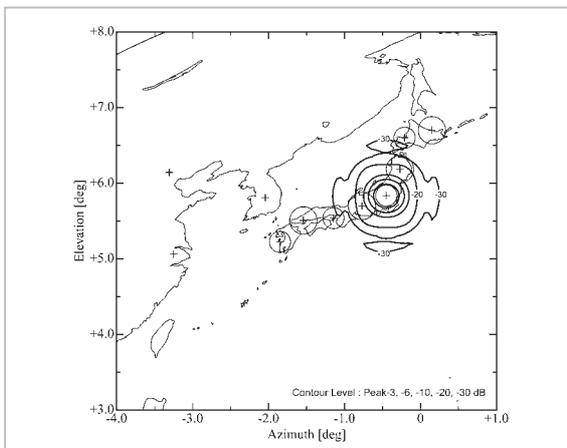
**Fig.4** Antenna Gain Contours of Kanto Beam (RX)
