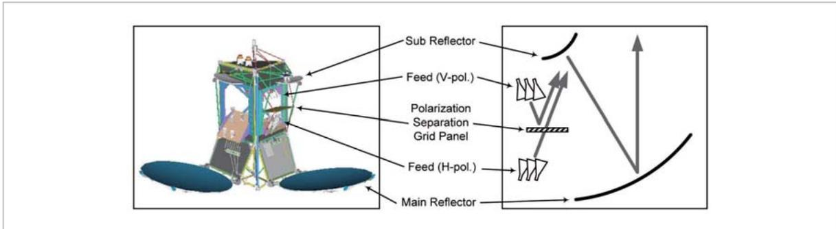
**Fig.2** Overview of Multi Beam Antenna
