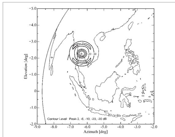
**Fig.6** Contours of Bangkok Beam (RX)
