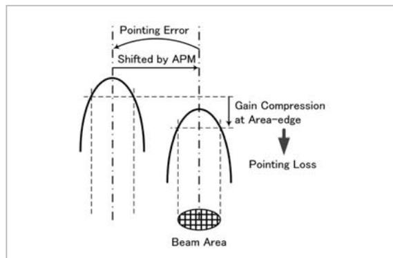
**Fig. 14** Pointing Loss caused by Beam Pointing Error
