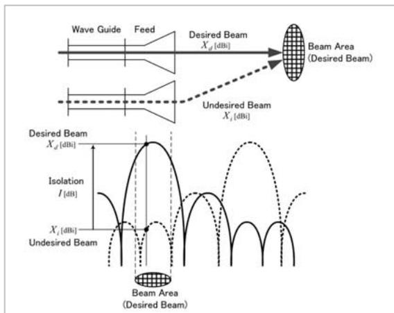
**Fig. 7** Isolation between each beams (TX)
