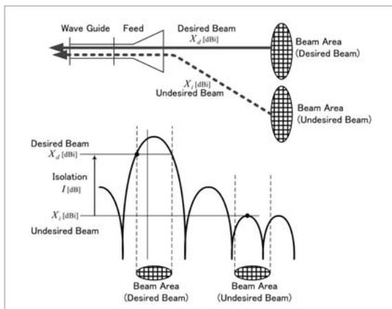
**Fig. 8** Isolation between each beams (RX)
