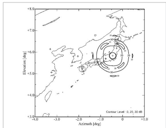
**Fig. 10** Analysis Result of Isolation (RX)
