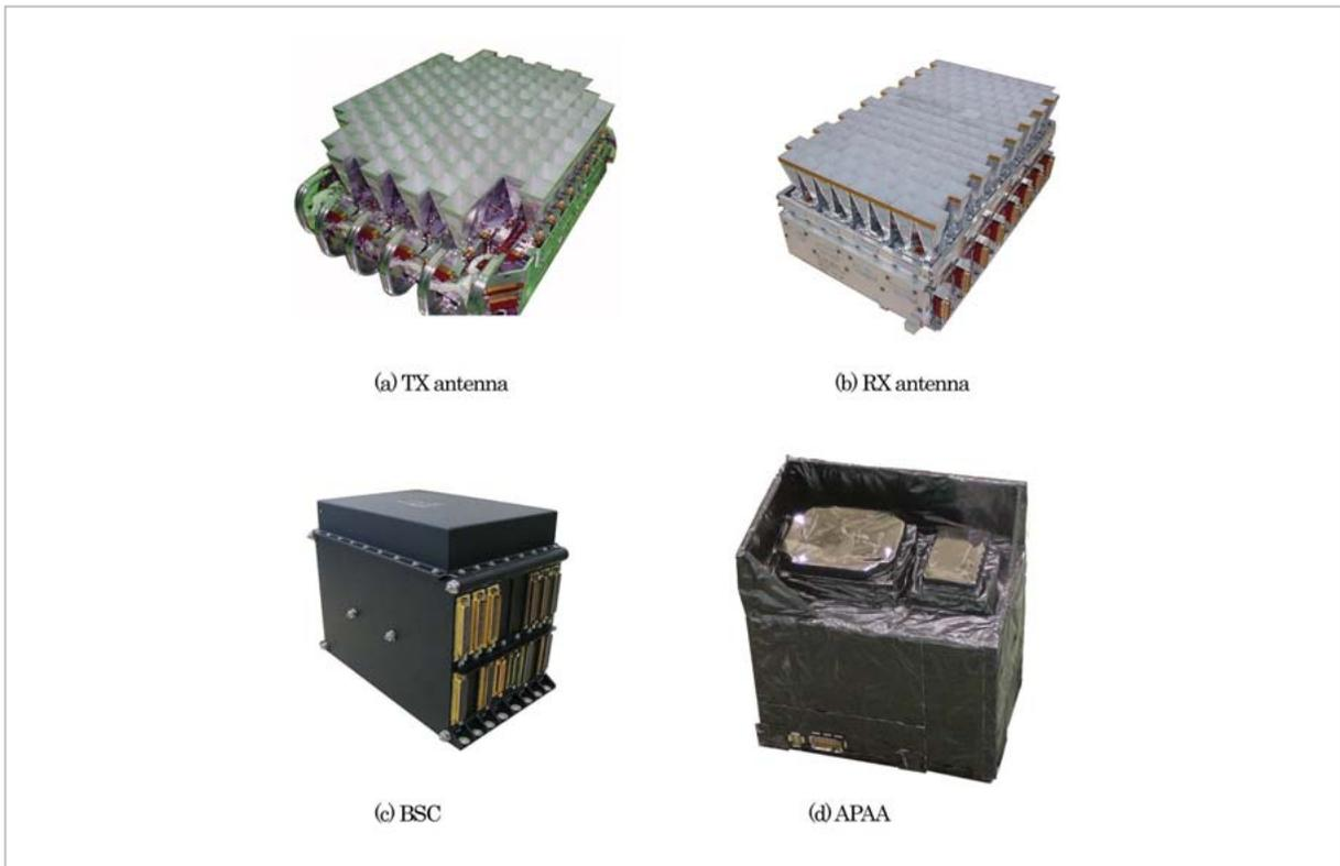
**Fig.6** Photos of the PFMs of the transmitting antenna, receiving antenna, BSC, and the APAA
